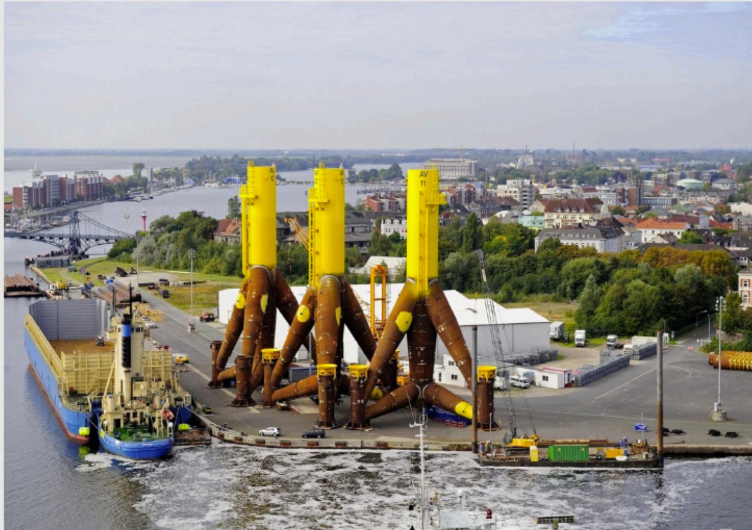
Fundaments for windmills for the windpark alpha ventus
