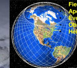
Field of view: ± 30°UV photonAperture diameter: 2.5 mEvent time sampling: 2.5 µs = 1 GTUObservational area: > 1.9 × 105 km²Height : 400 km
