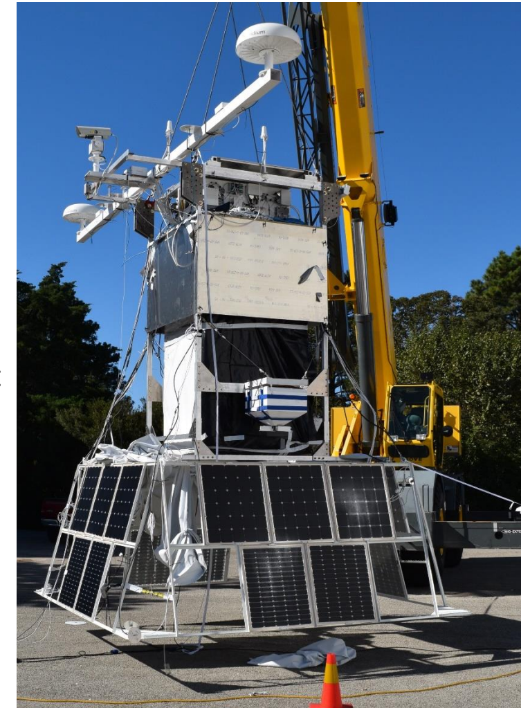
Euso-SPB during the hang test at the NASA CS-BS (Palestine-Texas)
