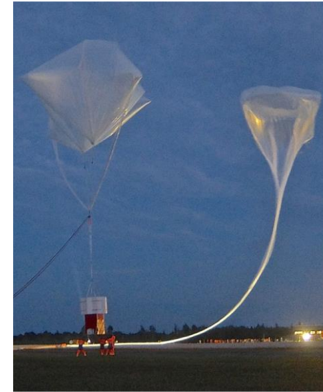
EUSO Balloon The first flying prototype of EUSO launched in 2014
