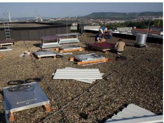
Detectors from KASCADE experiment have been placed on the roof of Sparkasse Versicherung building in Stuttgart. As a cosmic shower hits the roof, lights in the staircases flash and a skybeamer point in the direction of the shower.
