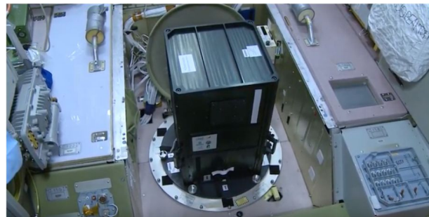
Mini-EUSO acquiring data on board of the ISS, screwed to a window of ZVEZDA module.
