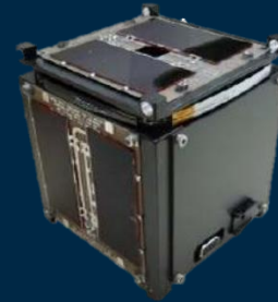
1U CubeSat CP1 (left) 10x10x11cm 3U CubeSat CP10 (right) 10x10x34cm (NASA)
