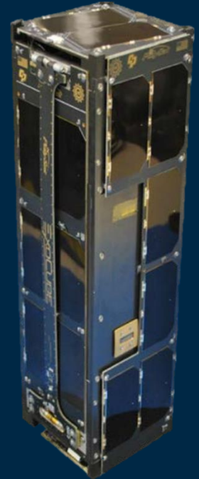
1U CubeSat CP1 (left) 10x10x11cm 3U CubeSat CP10 (right) 10x10x34cm (NASA)
