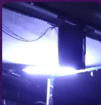
Background Light (2 strips of white LEDs)
