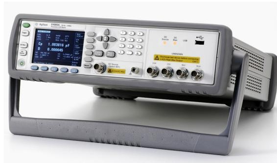
Figura 4.4: Agilent E4980A LCR Meter.
