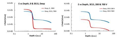
Fig. 8 Effect of irradiation on the electric field in the LGAD with deep gain layer: (left): pre-rad vs. high fluence with bias close to breakdown; (right): low bias vs. high bias for the "Deep" sensor heavily irradiated with neutrons to 3E15 Neq/ cm<sup>2</sup>.
