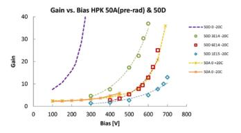
Fig.4 Gain-bias curves for HPK LGAD 50D and 50A pre-rad and 50D after neutron fluences of 3, 6,  $10*10^{14}$  Neq/cm<sup>2</sup>.
