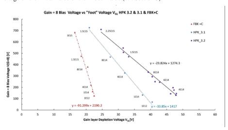
Fig. 10 Correlation between the bias for gain G=8, V(G=8), and the "Foot" voltage  $V_{GL}$  for the three selected sensors.
