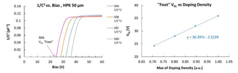
Fig.1 C-V analysis of the HPK prototype ECX20840 before radiation: (left): bias dependence of  $1/C^2$  to find the bias voltage  $V_{GL}$  which depletes the gain layer; (right): correlation between relative doping density and  $V_{GL}$ .
