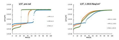
Fig. 5 Measured 1/C<sup>2</sup> vs. bias curves for three selected sensors (left): before irradiation; (right): after a neutron fluence of 1.5E15 Neq/cm<sup>2</sup>
