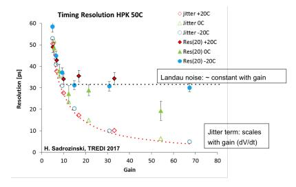
**Figure 2:** Variation of the jitter and total time resolution as a function of the UFSD gain, as measured on a Hamamatsu 50-micron thick UFSD sensor: the jitter term, calculated as  $\sigma_t(jitter) = N/(dV/dt)$ , decreases constantly with gain while the total time resolution flattens around  $\sigma_t(Total) = 30$  ps.
