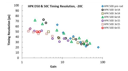
Figure 4: Time resolution evaluated at an optimized CFD fractions vs. gain for the different fluences at -20  $^{o}$ C.
