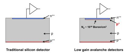
Figure 1: Schematic of a traditional silicon diode (left) and of a Low-Gain Avalanche Diode (right). The additional  $p^+$  layer underneath the  $n^{++}$  electrode creates, when depleted, a large electric field that generates charge multiplications.
