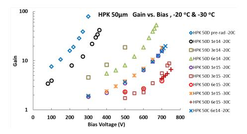
**Figure 3:** Gain as a function of bias of the LGAD irradiated to the indicated neutron fluences at  $-20 \,^{o}$ C and  $-30^{o}$ C, showing the need for increasing the bias of irradiated sensors to reach adequate gain.
