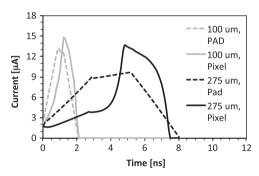
**Fig. 8.** Current signals as a function of time for 275  $\mu$ m and 100  $\mu$ m thick devices (pads vs. pixels, both with a gain of 15) simulated with the software Weightfield.
