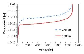
Fig. 3. Leakage current as a function of reverse voltage for  $100\,\mu m$  and  $275\,\mu m$  thick sensors.
