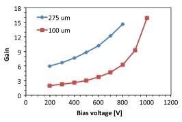
Fig. 5. Gain as a function of reverse voltage for 100  $\mu m$  and 275  $\mu m$  thick sensors. Data refer to the sensor response to a mip.
