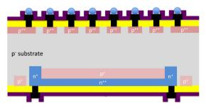
**Fig. 1.** Schematic cross section of proposed double-sided pixelated low gain avalanche detector (not to scale).
