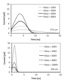
**Fig. 7.** Current signals as a function of time at different voltages: (top) 275  $\mu m$  thick device, and (bottom) 100  $\mu m$  thick device.
