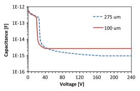
Fig. 4. Capacitance as a function of reverse voltage for  $100\,\mu m$  and  $275\,\mu m$  thick sensors.
