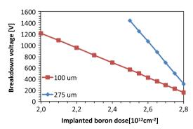
Fig. 2. Breakdown voltage as a function of the boron dose of the gain layer for  $100\,\mu m$  and  $275\,\mu m$  thick sensors.
