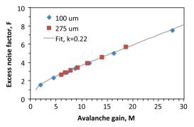
**Fig. 6.** Excess noise factor as a function of gain calculated analytically according to McIntyre's theory [16] for the two devices of different thickness, and fitting line of Eq. (1) for k=0.22.
