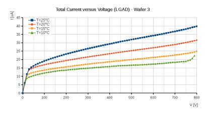
Figure 1. I-V curves at different temperatures in a LGAD with moderate gain ( $300\mu m$ , FBK).
