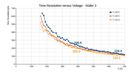
Figure 3. Time resolution for the moderate gain sensor at different temperatures ( $300\mu m$ , FBK).
