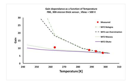
Figure 5. Gain as a function of temperature compared with simulation for  $300\mu m$  thick LGAD from FBK.
