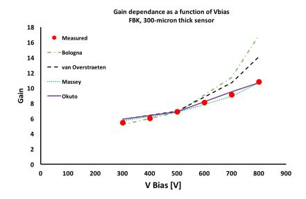
**Figure 4**. Gain at room temperature as a function of external voltage compared with simulation for  $300 \mu m$  thick LGAD from FBK.
