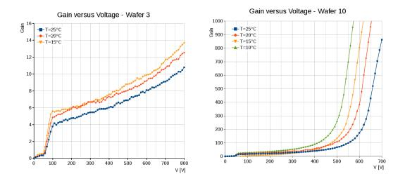
**Figure 2**. Gain as a function of bias voltage at different temperatures for a moderate gain (left) and high gain (right) device (both  $300\mu m$ , FBK).
