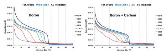
Fig. 2. – C(V) measurements performed on UFSD2 sensors: boron (left), boron with carbon (right).
