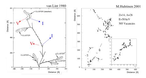
Figure 1: Spatial distribution of the damaged produced by a 1 MeV neutron in Silicon.
