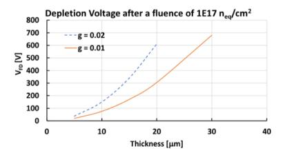
**Figure 3:** Depletion voltage after a fluence of  $1 \cdot 10^{17} n_{eq}/cm^2$  as a function of sensor thickness assuming a standard g = 0.02 or a saturated g = 0.01 value of the acceptor creation coefficient.
