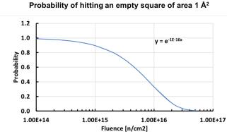
**Figure 2:** Probability as a function of particle fluence of hitting a square of  $1 \text{ Å}^2$  not previously hit by any other particle. As the probability decreases, saturation effects in Silicon damage are more likely.
