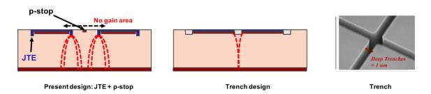
**Figure 8:** Left side: In the current LGAD design, the gain is terminated using junction termination extensions (JTE) and the n-doped pixels are isolated from each other using p-stops. This design creates a dead area between pads. In order to eliminate the dead area it has been proposed to use trenches to terminate the gain and isolate the pads.
