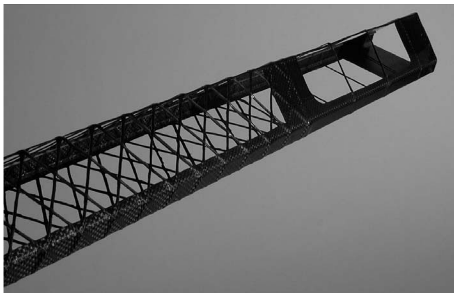
Figure 4.75: Ladder prototype produced to demonstrate the feasibility of the filament-winding technique.
