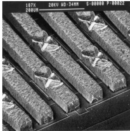
Figure 4.59: TAB bonded cable in staggered rows (courtesy of Bull/Dassault companies).
