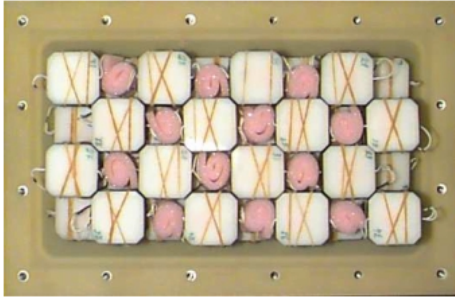
Figure 2.36: Arrangement of the 32 detector cells in two layers following a chessboard-like pattern.
