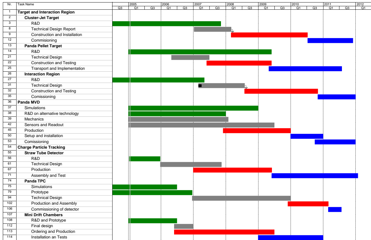
Figure 14.2: Work breakdown schedule for the interaction region (target, vertex detector), and the charged particle tracker of the PANDA detector.
