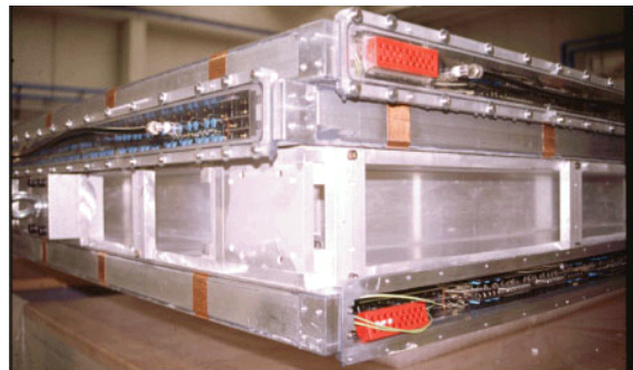
Figure 7.37: The photo of the full size prototype of the CMS DT chamber.
