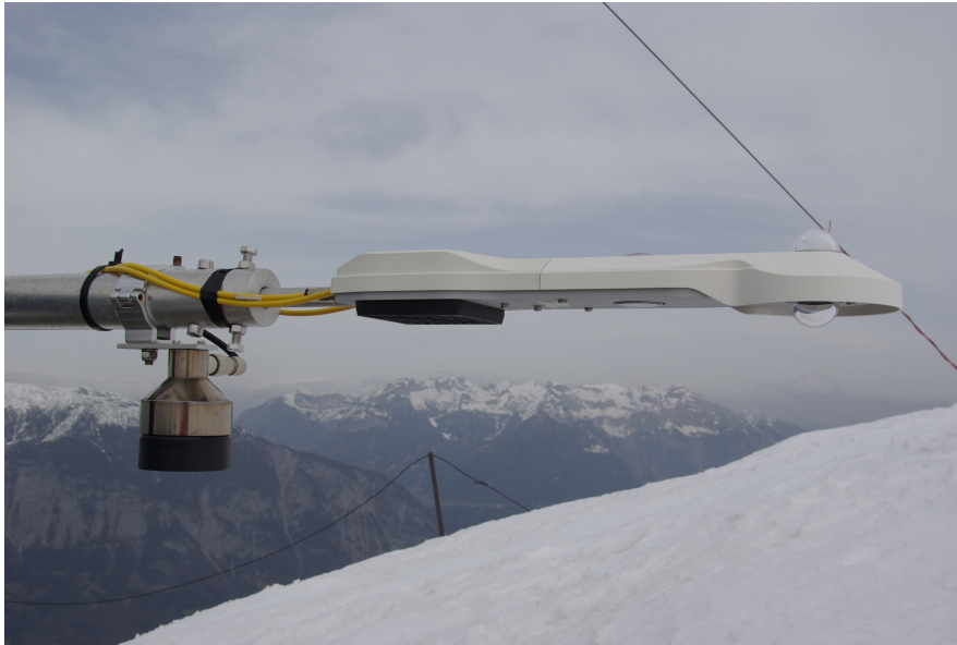
Figure 3.7: Arbeser station's CNR 4 Radiometer. It is possible to see the upper and lower plexiglass pyranometer domes, on the left there is the infrared snow sensor.
