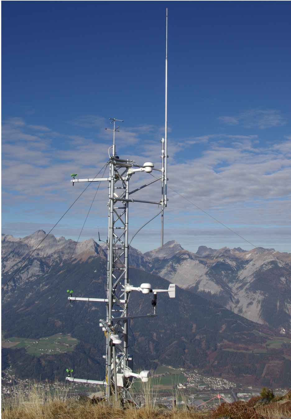
Figure 3.2: The Arbeser station mast, and we can clearly distinguish the three levels of cup anemometers and temperature/humidity measurements.
