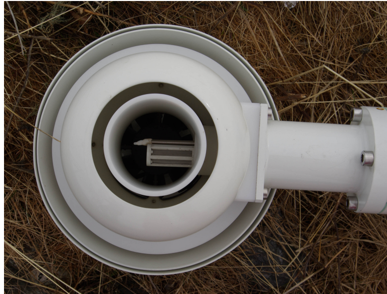
Figure 3.5: Rotronic temperature and humidity sensor inside the RS12T ventilated shield, it was unmounted on 1st April 2016 for routine maintenance of the station.
