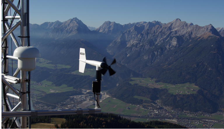
Figure 3.6: The Yuong wind monitor and the second temperature-humidity level (on the left) installed on the north side of Arbeser station; in the back ground the Inn Valley with Vomp village.
