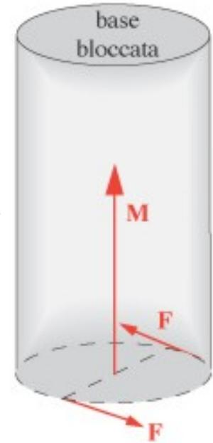
$$M = \frac{\pi}{2} G \frac{r^4}{l} \theta \quad \Rightarrow \quad M = k\theta \quad \text{Con:} \quad k = \frac{\pi}{2} G \frac{r^4}{l}$$
