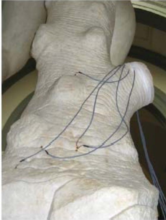
Fig. 23. (a) Strain gages disposition on the three trunk.
