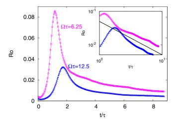
FIG. 4. Rossby number  $Ro = w_{rms}/(2\Omega h)$  as a function of time for the two rotations  $\Omega \tau = 6.25$  (pink circles) and  $\Omega \tau = 12.5$  (blue triangles). Inset: the same quantities in a log-log plot. The black line represents  $t^{-1}$  scaling.
