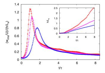
FIG. 3. Ratio of the vertical velocity fluctuations  $w_{\rm rms}$  to the width of the mixing layer h as a function of time for three different rotations,  $\Omega \tau = 0$  (red squares),  $\Omega \tau = 6.25$  (pink circles), and  $\Omega \tau = 12.5$  (blue triangles). Inset: time evolution of the mixing layer width h defined in terms of a threshold  $r\theta_0$  in the temperature profile, with r = 0.9.
