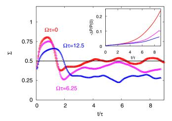
FIG. 5. Efficiency of kinetic energy production  $\Sigma = -(dE/dt)/(dP/dt)$  as a function of time for three different rotations,  $\Omega \tau = 0$  (red squares),  $\Omega \tau = 6.25$  (pink circles), and  $\Omega \tau = 12.5$  (blue triangles). Inset: potential energy loss  $-\Delta P(t) = P(0) - P(t)$  for the same three values of rotations (from top to bottom).
