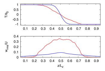
FIG. 7. Vertical profiles of mean temperature  $\overline{T}(z)$  (upper plot) and of vertical velocity  $\overline{w}_{rms}(z) = \overline{w^2}(z)^{1/2}$  for the simulation with  $\Omega \tau = 0$  (red lines) and  $\Omega \tau = 12.5$  (blue lines) at time  $t = 6\tau$ .
