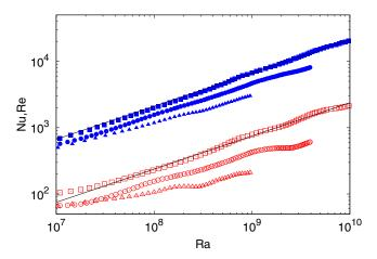
FIG. 8. Reynolds number (filled blue symbols) and Nusselt number (open red symbols) as a function of Rayleigh number for the simulations with  $\Omega \tau = 0$  (squares),  $\Omega \tau = 6.25$  (circles), and  $\Omega \tau = 12.5$  (triangles). The black lines represent the ultimate state behavior Ra<sup>1/2</sup>.
