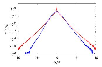
FIG. 10. PDF of vertical vorticity computed in the mixing layer of width h at time  $t = 3.2\tau$  for  $\Omega\tau = 0$  (red) and  $t = 5.6\tau$  for  $\Omega\tau = 12.5$  (blue). At these times the width of the mixing layer in the two cases is the same. The values of the vertical vorticity have been normalized with the standard deviation ( $\sigma = 0.010$  for  $\Omega\tau = 0$  and  $\sigma = 0.039$  for  $\Omega\tau = 12.5$ ).
