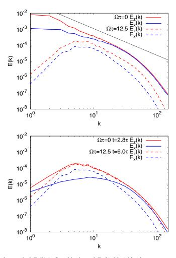
FIG. 9. Upper plot: vertical  $E_z(k)$  (red) and horizontal  $E_x(k)$  (blue) kinetic energy spectra computed at the time  $t=6.0\tau$  both in the absence of rotation (continuous lines) and with  $\Omega\tau=12.5$  (dashed lines). Lower plot: vertical and horizontal kinetic energy spectra computed at time  $t=2.8\tau$  for  $\Omega\tau=0$  and at time  $t=6.0\tau$  for  $\Omega\tau=12.5$  at which the peaks of the vertical spectra are the same.
