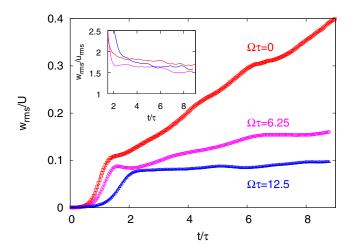
FIG. 2. Vertical velocity fluctuations  $w_{\rm rms}$  in the mixing layer as a function of time for three different rotations,  $\Omega \tau = 0$  (red squares),  $\Omega \tau = 6.25$  (pink circles), and  $\Omega \tau = 12.5$  (blue triangles). Inset: ratio of vertical to horizontal velocity fluctuations as a function of time, for the same values of rotation.
