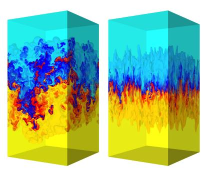
FIG. 1. Snapshots of the temperature field at time  $t = 5.2\tau$  for two simulations with  $\Omega\tau = 0$  (left) and  $\Omega\tau = 10$  (right) starting from the same initial conditions. Yellow (blue) represents hot (cold), light (heavy) fluid.
