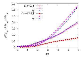
FIG. 6. Integral lengths based on the standard deviation of the fluctuation profile of temperature  $L^{(T)}$  (red squares), horizontal velocity  $L^{(u)}$  (pink circles), and vertical velocity  $L^{(w)}$  (blue triangles) without rotation (empty symbols) and for  $\Omega \tau = 12.5$  (filled symbols).
