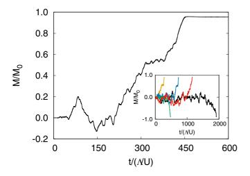
FIG. 3. Temporal evolution of the angular momentum *M* normalized with  $M_0 = \frac{2}{3}UR$  for the simulation at  $R = 31\Lambda$  and  $\alpha = -1.75$ . The inset shows the evolution of the angular momentum for an ensemble of simulation with different initial conditions with  $\alpha = -1.50$  and  $R = 16\Lambda$ .
