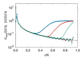
FIG. 6. Radial profiles of the vorticity,  $\overline{\omega}(r)$  (empty symbols), and of the rms vorticity,  $\overline{\omega}_{\rm rms}(r)$  (filled symbols), for simulations with  $R = 31\Lambda$ ,  $\alpha = -1.5$  (blue squares),  $\alpha = -1.75$  (red circles), and  $\alpha = -2$  (green triangles). The black line is the prediction  $|\overline{\omega}(r)| = U/r$ .
