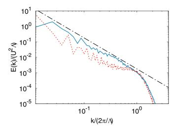
FIG. 4. Energy spectra for the simulation with  $R = 31\Lambda$  and  $\alpha = -1.75$  at  $t = 210\Lambda/U$  (blue, solid line) and  $t = 550\Lambda/U$  (red, dashed line). The black, dash-dotted line represents the slope  $k^{-2}$ .
