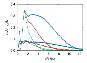
FIG. 7. Radial profiles of the radial and tangential components of the velocity fluctuations,  $\overline{u'_r}(r)$  (empty symbols) and  $\overline{u'_{\varphi}}((r)$  (filled symbols), as a function of the distance from the boundary for  $\alpha = -1.75$ ,  $R = 31\Lambda$  (blue squares),  $\alpha = -1.5$ ,  $R = 23\Lambda$  (red circles), and  $\alpha = -1.25$ ,  $R = 16\Lambda$  (green triangles).
