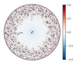
FIG. 9. Vorticity field in late stage of the simulation with  $R = 31\Lambda$  and  $\alpha = -1.50$ , which displays a giant vortex whose core consists of a binary rotating system of two small, equal-sign vortices.
